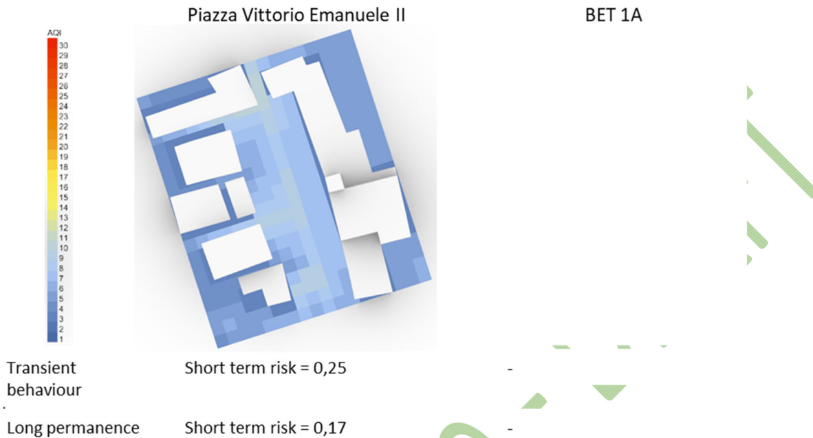
Figure 6. Comparison of air pollution risk conditions in the pre-mitigation scenario of Piazza Vittorio Emanuele II and reference BET 1A (for air pollution risk the AQI analyses for BET are not available)
