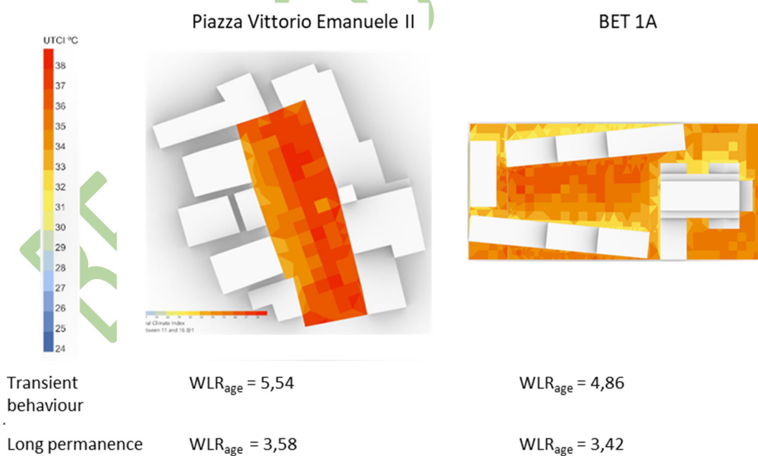
Figure 7. Comparison of heatwave risk conditions in the pre-mitigation scenario of Piazza Vittorio Emanuele II and reference BET 1A.
